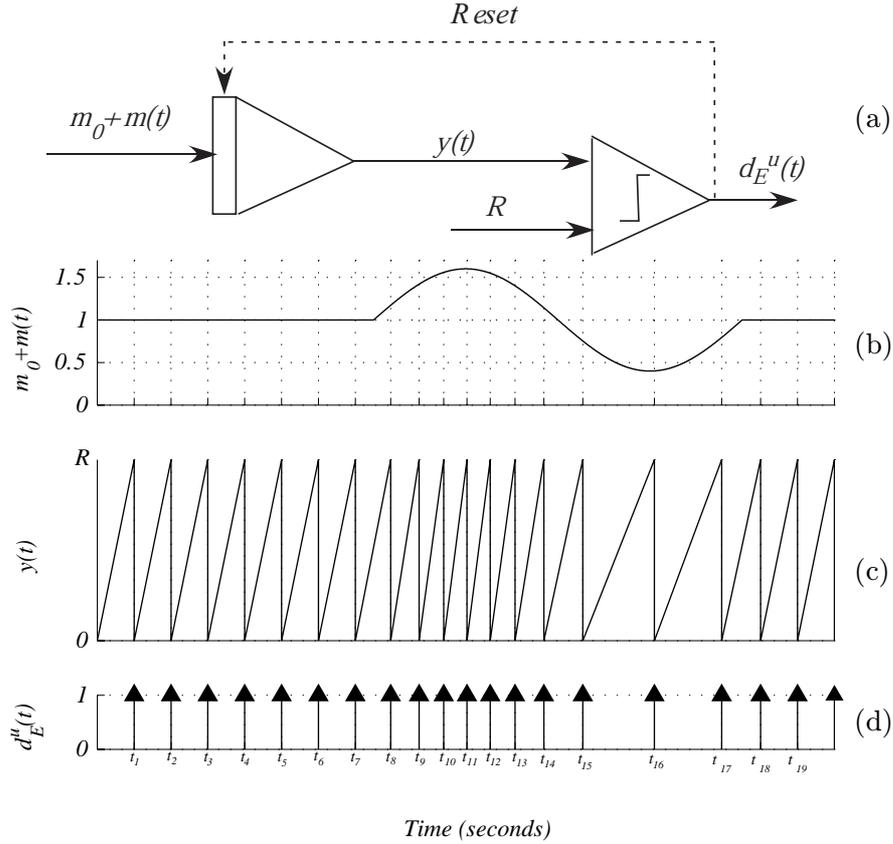
Figure 2: (a) The integral pulse frequency modulation model, (b) the input signal  $m(t)$  which modulates the variations in interval length, (c) the output of the integrator assuming a threshold level at  $R$ , and (d) the resulting event series at times  $t_0, t_1, \dots$
